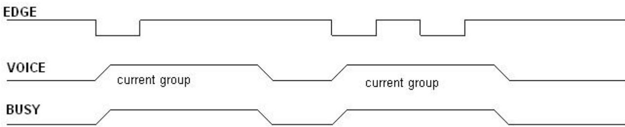
Remark: Edge trigger. When I/O test falling edge( such as this I/O short touch GND) ,the voice will be triggered. During the playing , the next falling edge will not interrupt the voice,after voice play finished,falling edge will make it replay .
