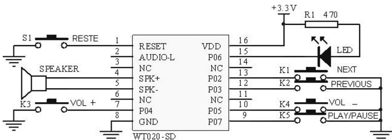
WTV020-SD-16P and WTV020-SD-20S, In PWM output, SPK+ ,SPK- connect to speaker .
