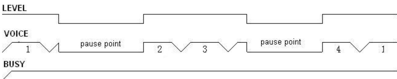
Negative level trigger. Power on , it will play automatically, negative level trigger P05 to pause , next tirgger to play from the pause point. After voices play finished, it will loop .
